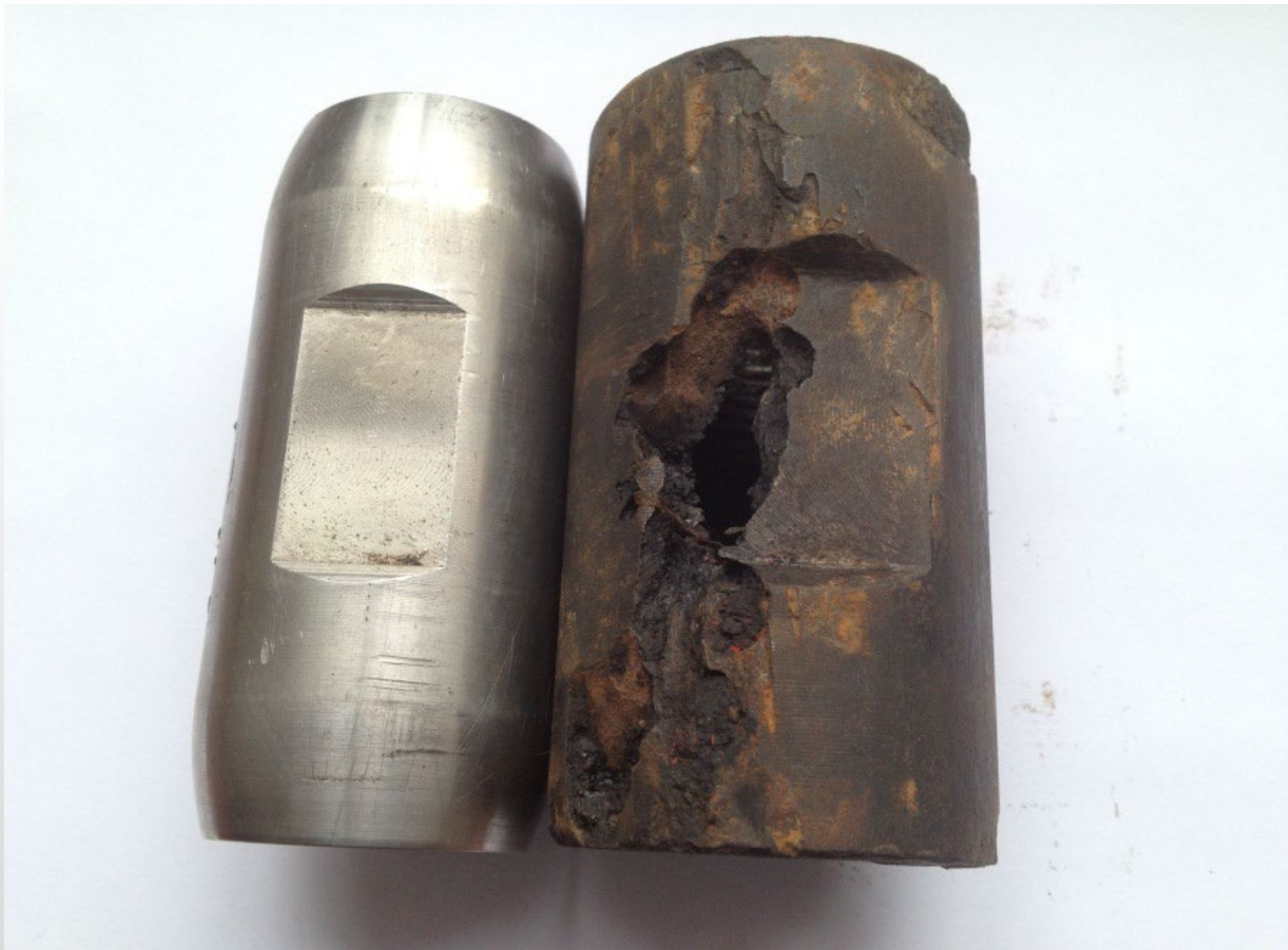
Comparison between super stainless steel and ordinary oil field steel (coupling) after 280 days of working underground in Sinopec Shandong Oilfield
